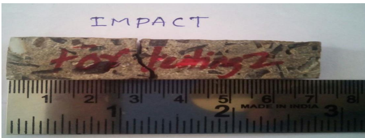
Fig. 4 Cracked DRFP composite specimen under impact test.
