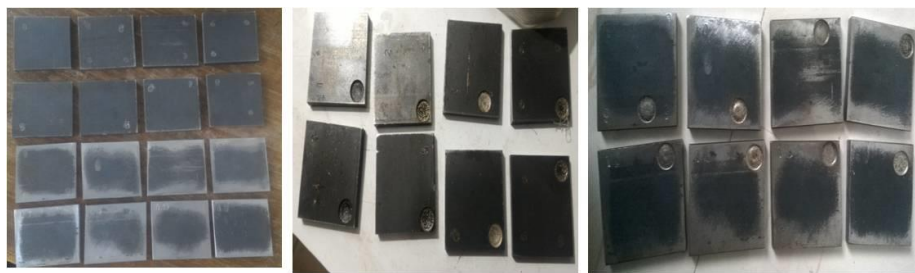
Figure 1: Samples before and after machining with both the tools
