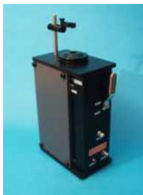
Fig 3 Dantec Dynamics hot wire calibrator
