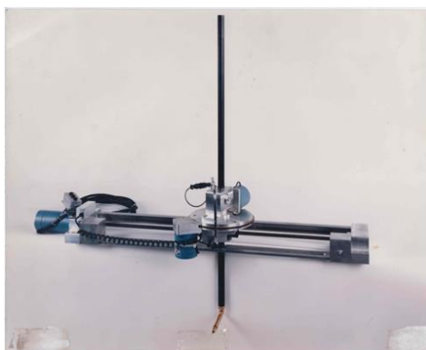
Fig 4 Aerolab Probe Traverse mechanism
